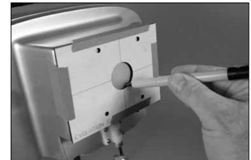
Tape the engine mounting template to the firewall. Mark the location for the cutout for the fuel tank neck on the firewall.
