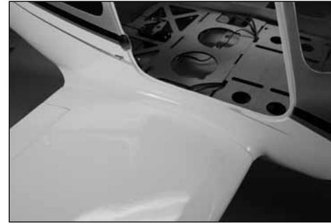
Slide the wing into position, guiding the leads for the flap and aileron into the fuselage. Connect the leads, then use the wing bolt to secure the wing to the fuselage.
