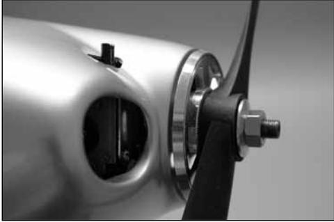
Slide the cowling into position. Trim the cowling to clear the nose gear and the carburetor when a gas engine has been installed. Slide the spinner backplate on the engine shaft, then the propeller. Secure the propeller to hold the backplate in position. Set a 3/32-inch (2mm) gap between the cowl and spinner, then tape the cowl to the fuselage.
