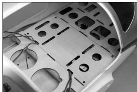
Secure the cover in the fuselage by installing the four screws removed in step 1. The flap and aileron leads will exit the notches in the tray so the leads from the wing can be plugged in.
