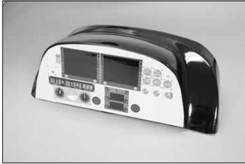
Use hobby scissors to trim the instrument panel to fit into the fuselage. Apply the instrument panel decal to aid in trimming the bottom edge of the instrument panel.
