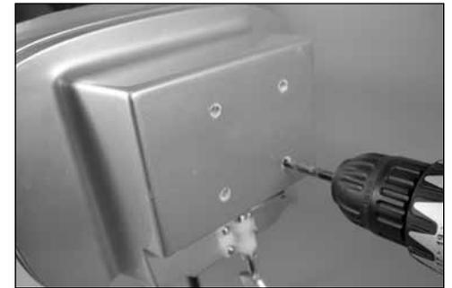
Remove the template from the firewall. Use a drill and 7/32-inch (4mm) drill bit to enlarge the holes in the firewall.
