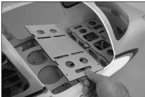
Remove the four screws holding the plywood cover inside the fuselage. Lift the tray and set it aside.
