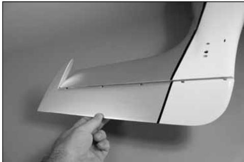
Slowly work the rudder into position. Use care not to force the rudder, as it could break the balance tab from the rudder.
