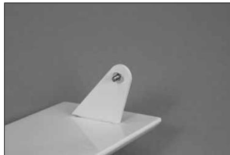
Insert the M3 x 8 socket head screws into the hinge, then slide an M3 washer on the screw. Note that the heads of the screws will face toward the wing tip when the flap is installed.
