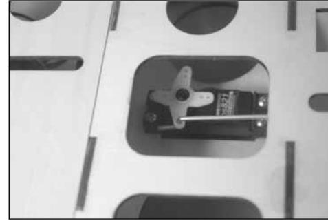
Fit the steering pushrod back into the fuselage, this time from inside the fuselage. Attach the clevis to the steering arm, then secure the servo arm to the steering servo. Adjust the clevis as necessary so the nose wheel is centered when the servo is centered. Slide the retainer over the forks of the clevis to keep it secure to the arm.
