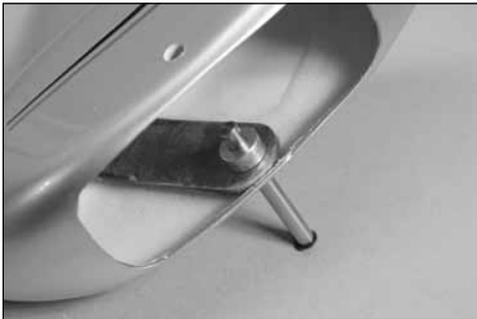
Slide the axle into position, then place a wheel collar on the axle.
