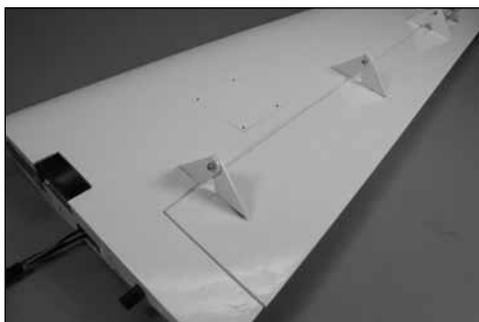
While holding the cover away from the wing slightly, turn on the radio system. Move the flap switch to the UP position, then check the fit of the cover to the wing. When the cover is in position, the flap will be in the UP position. Adjust the linkage as necessary to set the linkage length. Once set, tighten the nuts against the clevises and slide the tubing over the forks of the clevises.
