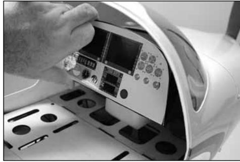
Fit the instrument panel into the fuselage. Use silicone adhesive to glue the instrument panel into the fuselage.
