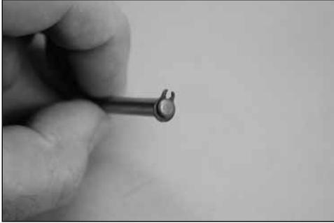
Use snap ring pliers to attach a snap ring to one end of the nose gear axle.
