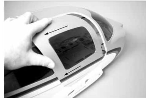
Slide the door latches rearward to release the doors from the fuselage. The front of the doors are not hinged to the fuselage. Simply slide the door rearward and remove it from the fuselage.
