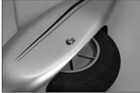
Fit the wheel in the wheel pant, then slide the axle through the wheel. Before sliding the axle through the opposite side of the wheel pant, slide a wheel collar on the axle. Once the axle is in position, attach the second snap ring to secure the axle.
