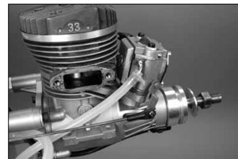
Secure the line from the clunk to the carburetor. The line from the vent is routed to the bottom of the fuselage. The remaining line will be used to fuel the model and will use a fuel dot mounted to the side of the cowling later in the manual.
