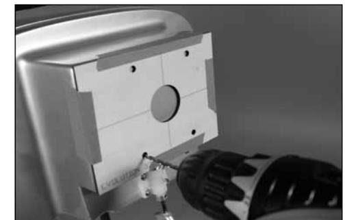
Use a drill and 1/16-inch (1.5 mm) drill bit to drill the pilot holes for your particular engine.
