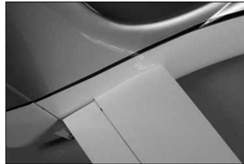
Place the remaining stabilizer in position on the joiner rods.
