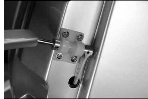
Slide a wheel collar on the nose gear wire. Insert the wire through the bracket, then place the steering arm on the wire. The top of the wire will be flush with the top of the steering arm. Slide the wheel collar against the bracket to keep the nose gear from moving up or down.
