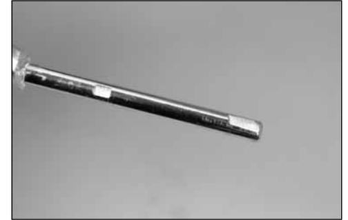
Remove the steering arm and wheel collar from the nose gear wire. Use a flat file to make flat areas on the nose gear where the setscrews left marks on the wire.
