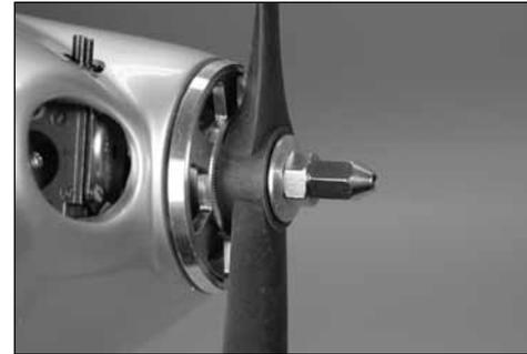
Reattach the backplate and propeller. The spinner adapter can be installed at this time. Make sure to use a box wrench when tightening the nuts.
