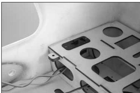
Mount the switch in the fuselage using the hardware provided with the switch.
