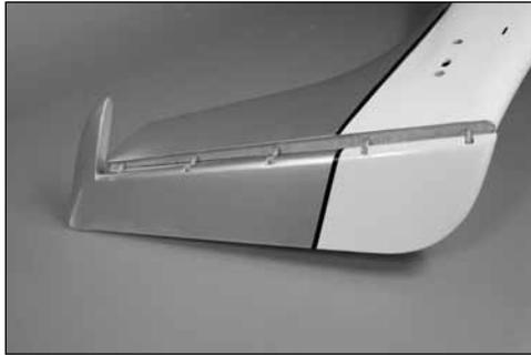
Fit the rudder to the fin. The rudder will need to be deflected as shown to get the hinges to align and still clear the balance tab.
