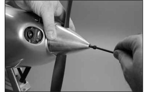
Attach the spinner to the engine. Make sure the spinner cutouts do not contact the propeller blades.
