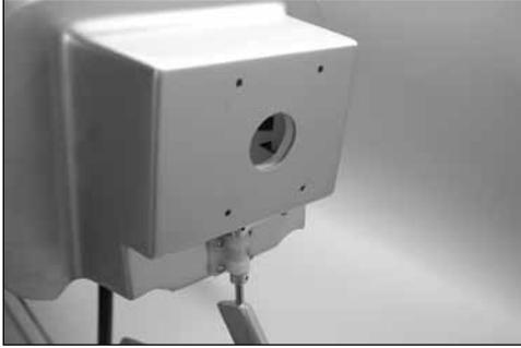
Remove the template from the firewall. Enlarge the holes for the engine mounting screws using a drill and 7/32-inch (4mm) drill bit. Make the opening for the fuel tank using a rotary tool and sanding drum.
