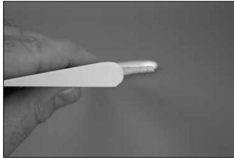
Position the hinge so the pin is aligned with the center of the leading edge radius. Each hinge must be positioned individually, as the radius changes along the length of the control surface.
