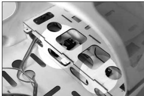
Install the steering servo in the fuselage next to the receiver switch with the servo shaft facing the rear of the fuselage. Make sure to prepare the servo mounting holes by threading the servo mounting screw into each hole, then hardening the holes using thin CA.
