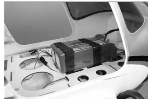
Use hook and loop straps (not included) to secure the batteries inside the fuselage. Place hook and loop tape (not included) between the batteries and cockpit floor to keep the batteries from sliding during flight. Use an EC5™ series battery connector to connect the batteries to the speed control.
