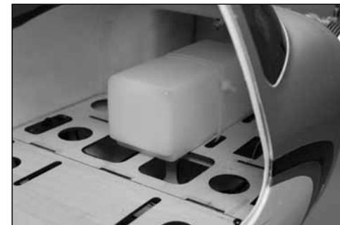
Insert the tank into the fuselage, guiding the tubing through the hole in the firewall. The fuel tank is secured using tie wraps (not included).
