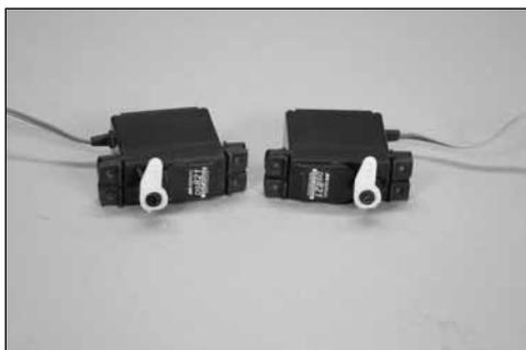
Prepare the aileron servos by installing the grommets and eyelets. Center the servos using the radio system and install the servo arms so they are perpendicular to the servo center line. The clevis for the aileron linkage will attach to the hole that is 19/32 inch (15mm) from the center of the servo arm.
